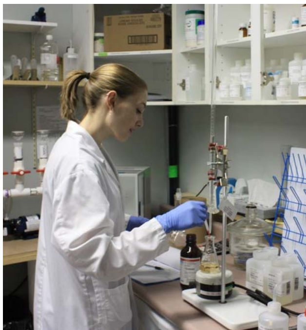
Laboratory Technician Jenine Bin titrates some water samples for Alkalinity at Central Labs.
